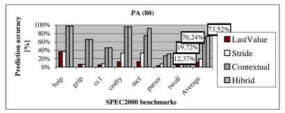
Figure 8: Prediction accuracy using 16 favorable registers (SPEC 2000)
