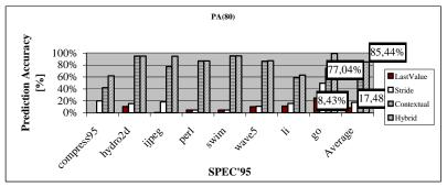
Figure 7: Prediction accuracy using 8 favorable registers (SPEC'95)
