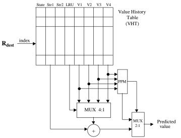
Figure 6: The hybrid predictor (context-based & stride)
